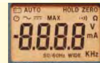
Backlit 10 000 counts LCD screen
